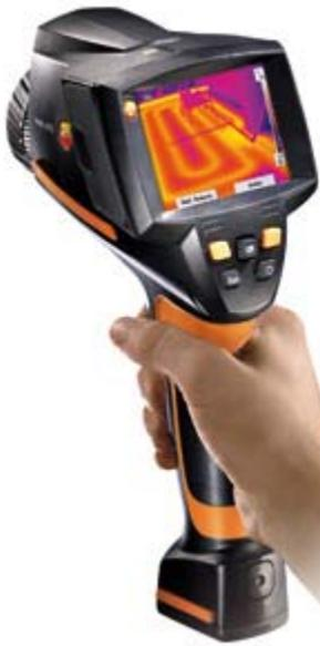
The thermal imager 875 is a reliable, solid tool for daily use. With a temperature resolution of < 80 mK, exchangeable lenses and an integrated digital camera, you can trace pipes and identify areas of water damage, discover weak spots in buildings quickly and simply
