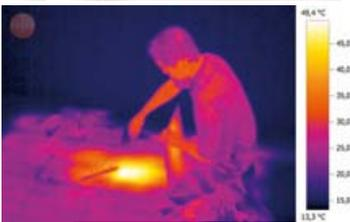
**Special measurement mode for detecting areas with danger of mould** Using the externally measured ambient temperature and air humidity, as well as the surface temperature, the humidity value of each measurement point is calculated and shown in the display as a real humidity image.
